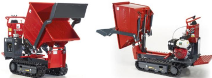
◀ The tipping mechanism with hydraulic cylinder makes it possible to unload the material or partialize the unloading operation according to the needs.
