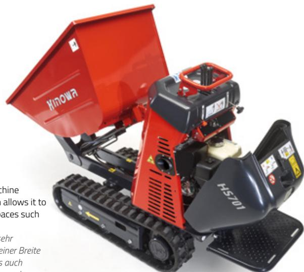
◀ It is a very compact machine at 758 mm width which allows it to pass through narrow spaces such as doors and gates.
