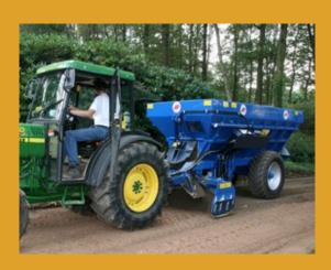
The AP leveldumper is a perfect machine for building and maintening of dirt roads, cycle paths, walking paths, entrances etc. This machine makes it possible to optimally spread all sorts of pavement material. The working width is infinitely variable by hydraulic cylinders.
