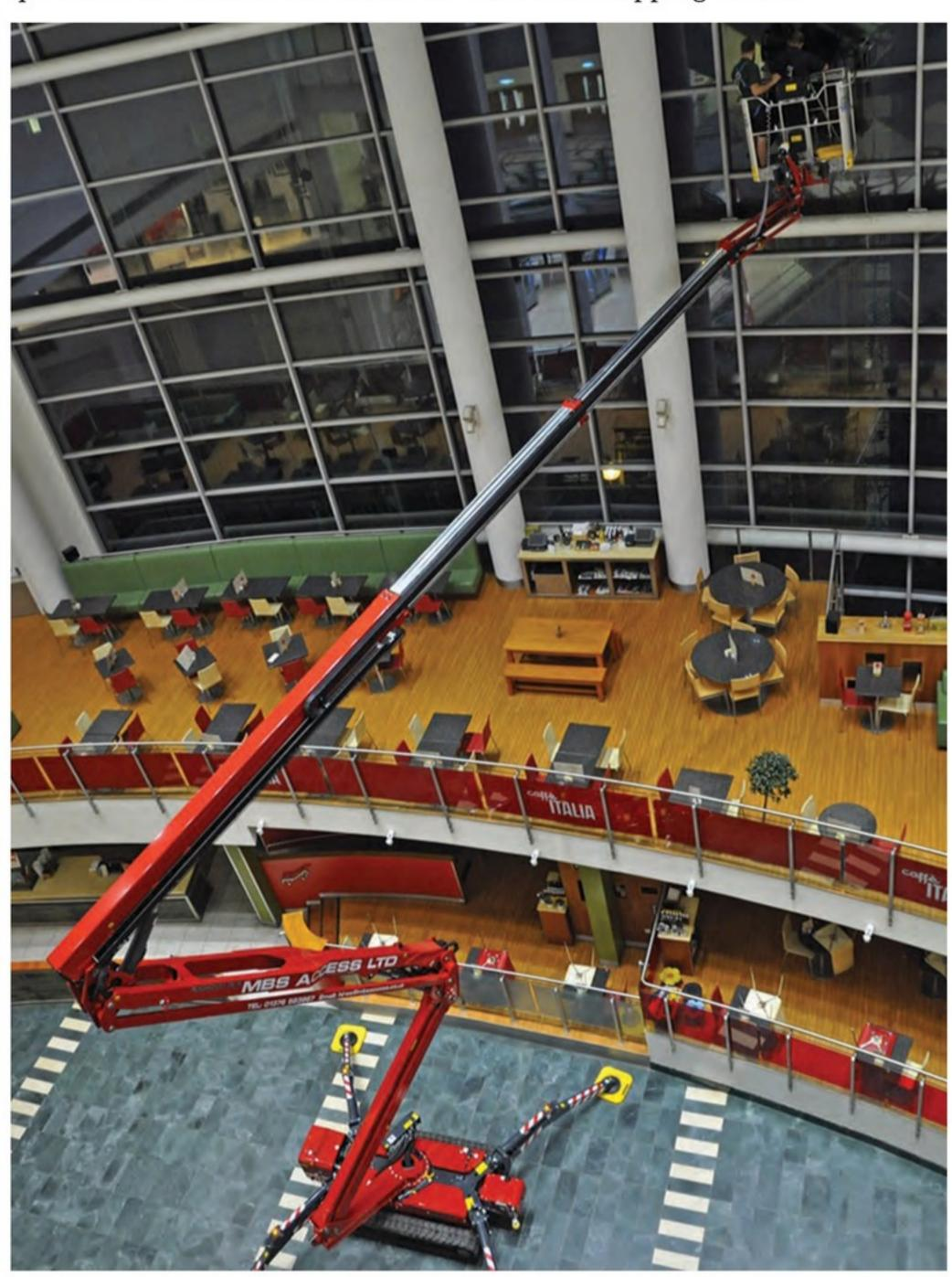
230kg – enough for two people with tools – without restriction throughout its entire working envelope. The dual pantograph boom design enables working flush with walls and the drive
